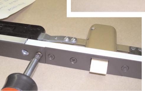
Install (3) 8-32 X 3/8" FHMS through the face-plate and into the aluminum "I" Beam, guide bar assembly. HAND TIGHTEN these screws to prevent stripping.
