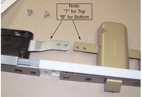
Locate the Top and Bottom Modules, they are different and are marked accordingly.
