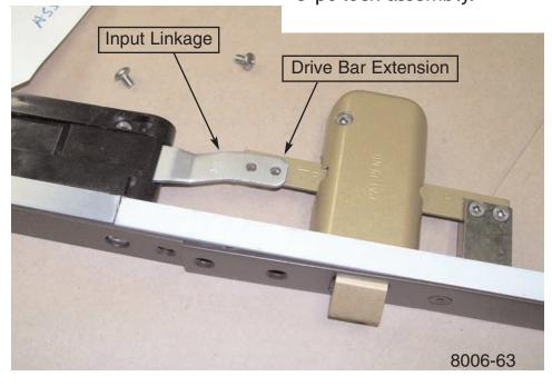
Install (2) 8-32 X 1/4" PHMS through the aluminum input linkage and into the gold drive bar extension. HAND TIGHTEN these screws to prevent stripping.
