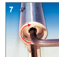
7 Make adjustment at bottom with 4 mm Allen key.
