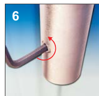
6 Loosen the set screw with 2,5 mm Allen key.
