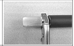
2. Use the provided fasteners and install one of the screws so it pierces through both the rail and connector. Pre-drilling is recommended. (This secures the connector in place to prevent from sliding when installing the next joining piece of ADA rail). Install screws on what will be the underside of the installed rail so they will not be visible. Screw heads can be painted with touch up paint to further conceal them.
